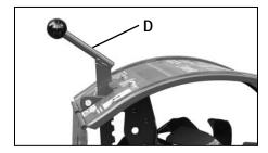
Figure 3-2: Depth Regulator Lever.
